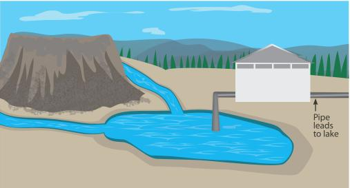
In the treatment plant, the mine water goes through a mixing and filtering process which reduces the levels of elements, such as Selenium and Copper, in the water.
