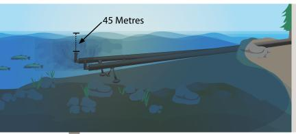
The treated water is sent through a pipe to Quesnel Lake at a depth of 45 metres and 250 metres away from the shore where it is diluted by mixing with lake water as fast as possible.
